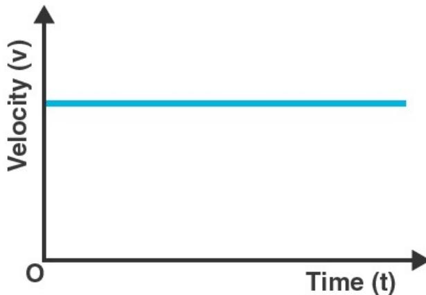
Since there is no change in the velocity of the object (Y-Axis value) at any point of time (X-axis value), the object is said to be in uniform motion.
