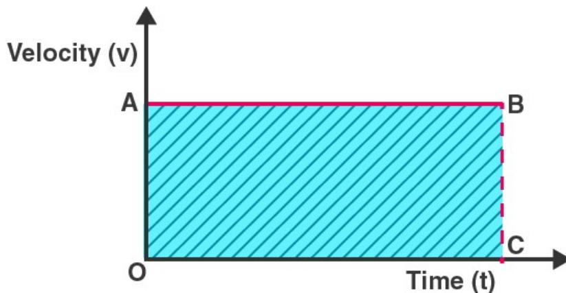
Now, the area below the velocity-time graph is the area of the rectangle OABC, which is given by  $OA \times OC$ . But OA is the velocity of the object and OC represents time. Therefore, the shaded area can be represented as:
