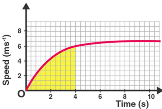
The shaded area represents the displacement of the car over a time period of 4 seconds. It can be calculated as:
