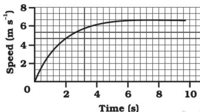
(a) Find how far does the car travel in the first 4 seconds. Shade the area on the graph that represents the distance travelled by the car during the period.
