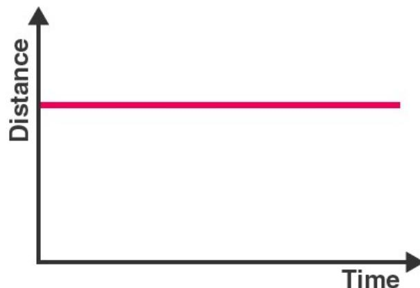
When the slope of the distance-time graph is a straight line parallel to the time axis, the object is at the same position as time passes. That means the object is at rest.
