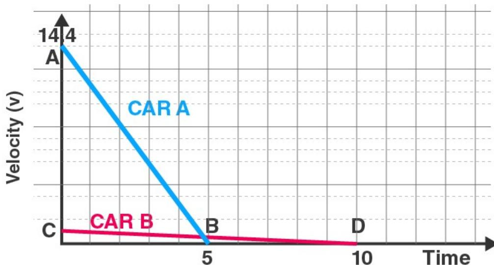
The total displacement of each car can be obtained by calculating the area beneath the speed-time graph.
